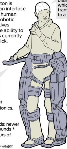
**2. The computer translates the brain activity and sends a signal to the exoskeleton, guiding the device without using the joystick**
